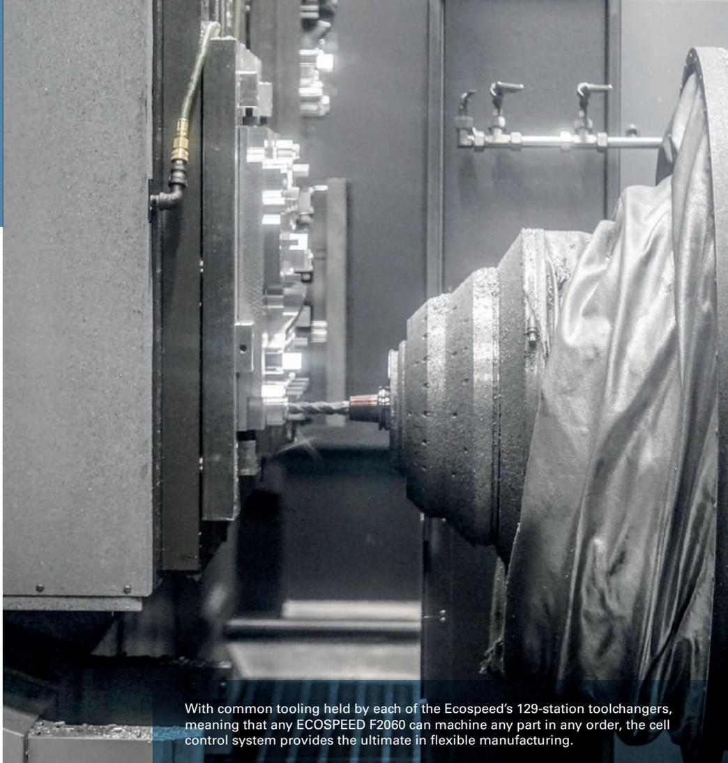
With common tooling held by each of the Ecospeed's 129-station toolchangers, meaning that any ECOSPEED F2060 can machine any part in any order, the cell control system provides the ultimate in flexible manufacturing.
