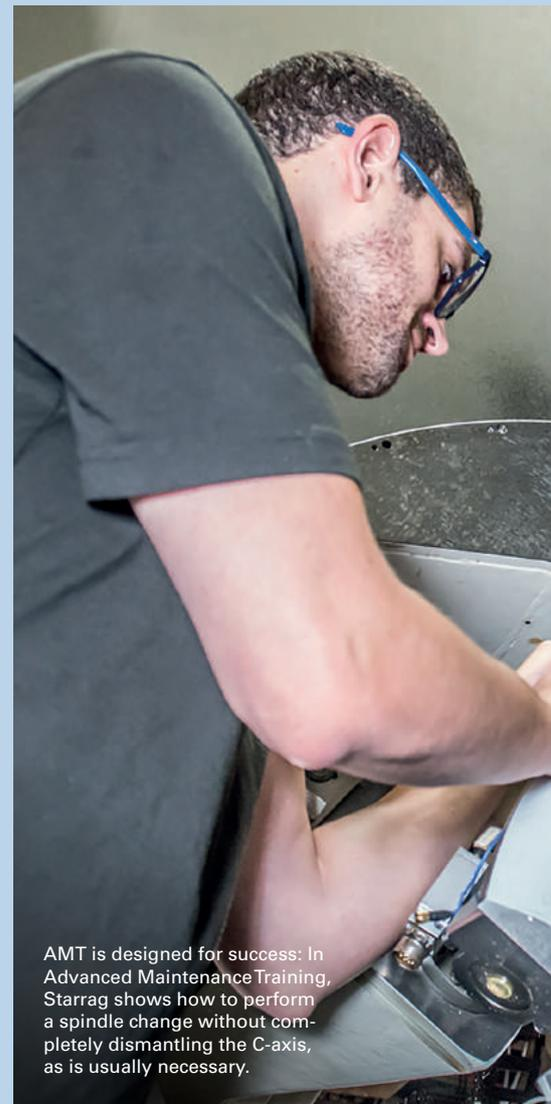
AMT is designed for success: In Advanced Maintenance Training, Starrag shows how to perform a spindle change without completely dismantling the C-axis, as is usually necessary.
