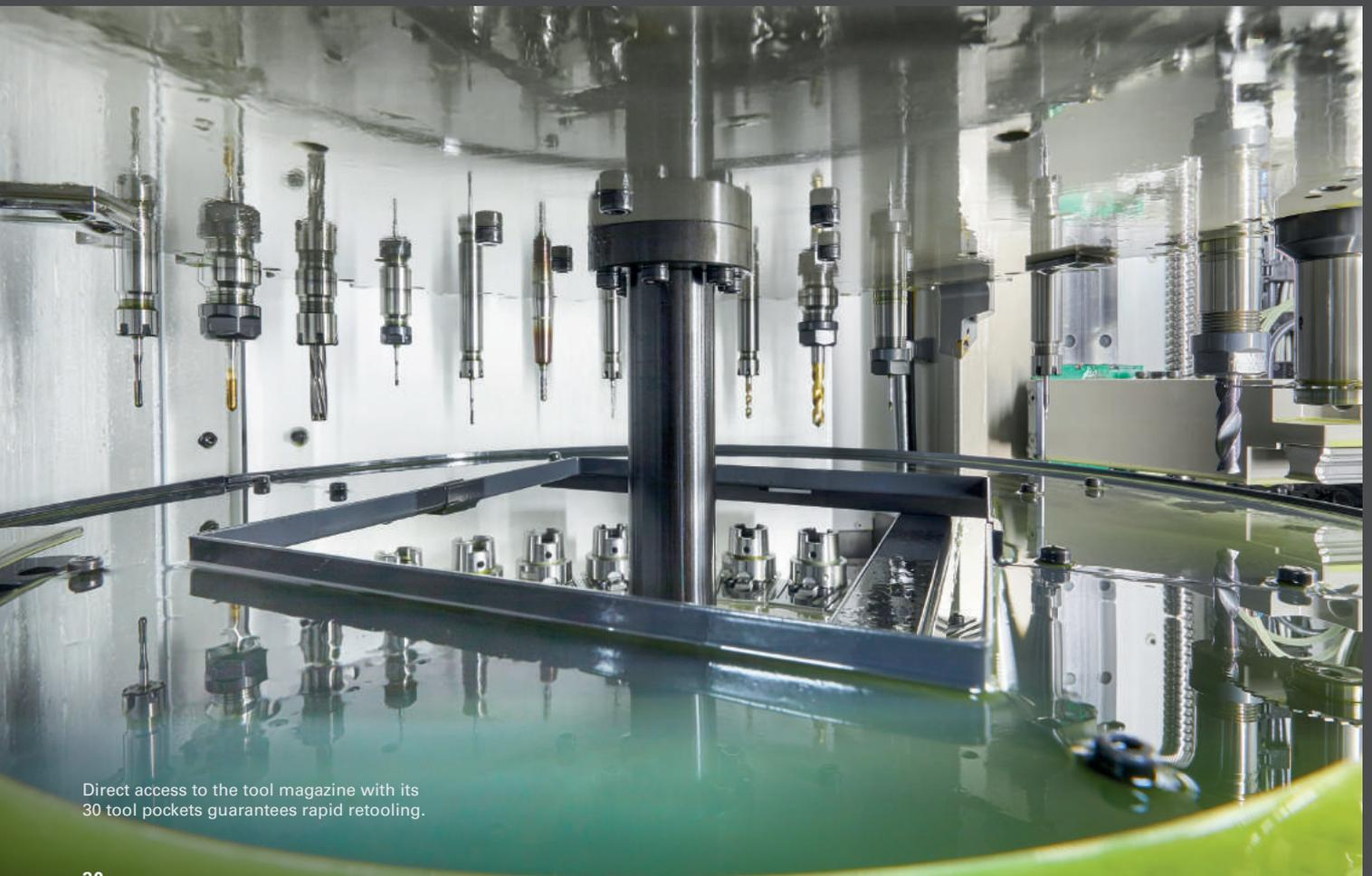
Direct access to the tool magazine with its 30 tool pockets guarantees rapid retooling.
