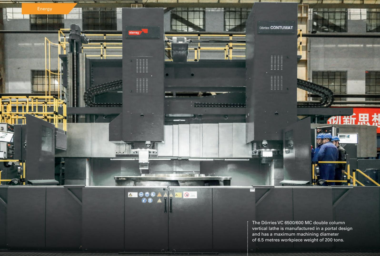
The Dörries VC 6500/600 MC double column vertical lathe is manufactured in a portal design and has a maximum machining diameter of 6.5 metres workpiece weight of 200 tons.
