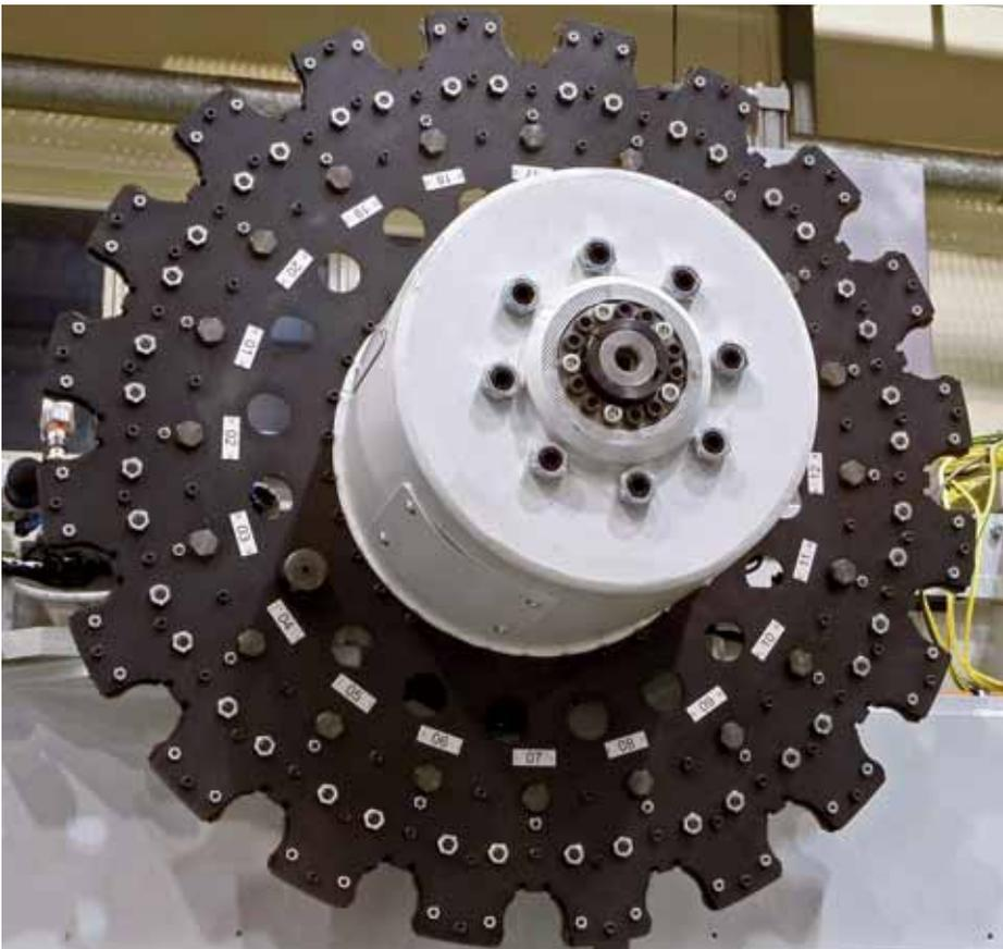
“From the circular tool magazine with 20 slots to the linear magazine, the machine can be individually equipped with 320 tools.”
