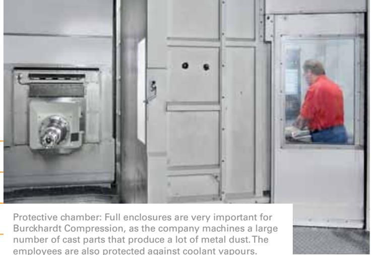
Protective chamber: Full enclosures are very important for Burckhardt Compression, as the company machines a large number of cast parts that produce a lot of metal dust. The employees are also protected against coolant vapours.
