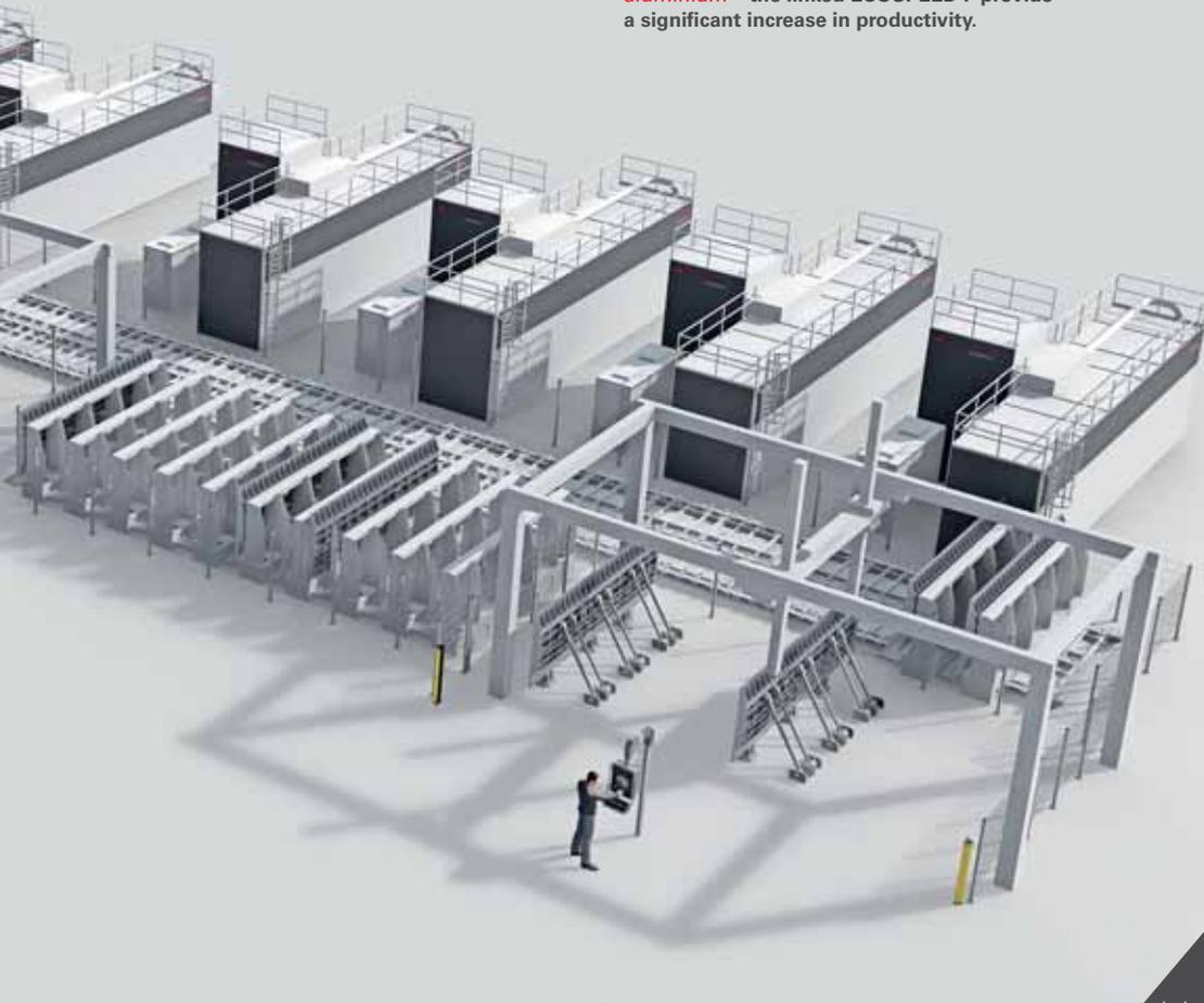
If a customer operates at the final stage of expansion, all they need to do is feed the parts for processing into a material accumulator. The rest happens fully automatically: from loading and storing the raw material, to various machining steps and, finally, to unloading the finished workpieces. All the data and resources are managed by the cell controller, which receives the orders directly from the end customer's ERP (Enterprise Resource Planning) system.
