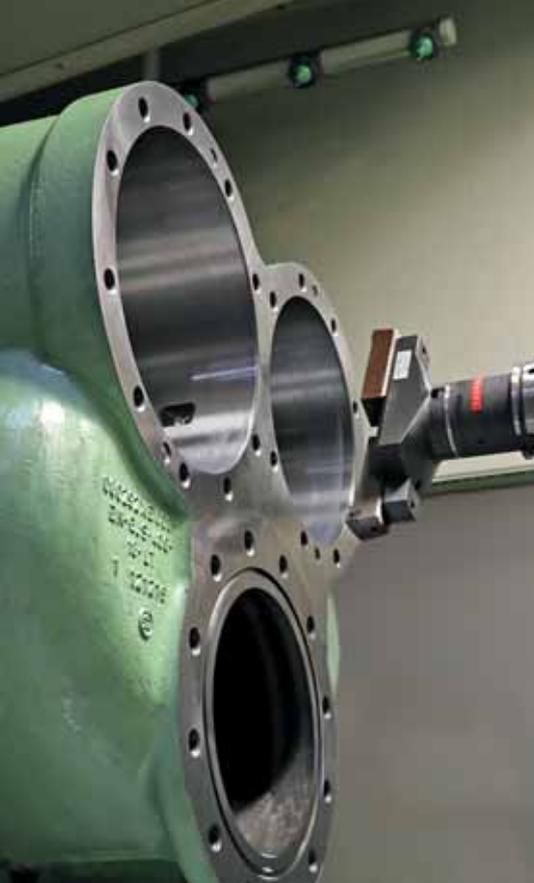
Important advantages of the Heckert HEC 630 and HEC 800 machining centres: large working area and quills for creating deep bore holes with high process reliability.
