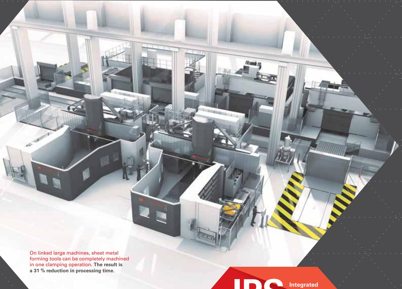
On linked large machines, sheet metal forming tools can be completely machined in one clamping operation. The result is a 31 % reduction in processing time.
