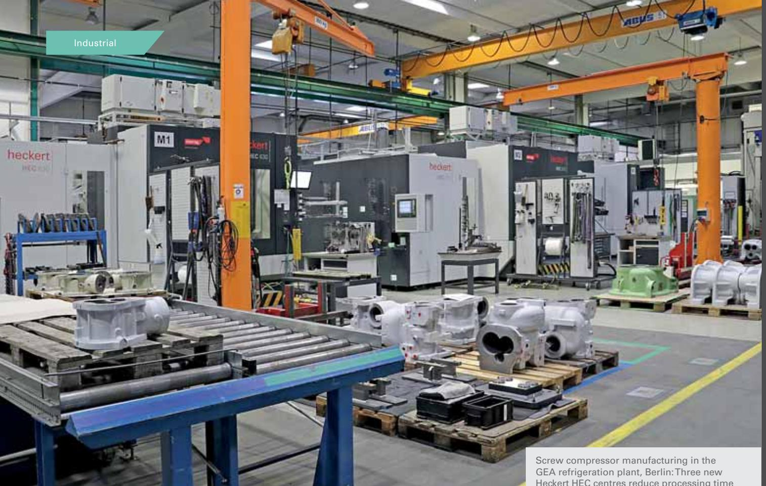
Screw compressor manufacturing in the GEA refrigeration plant, Berlin: Three new Heckert HEC centres reduce processing time for housing units by around 40%.
