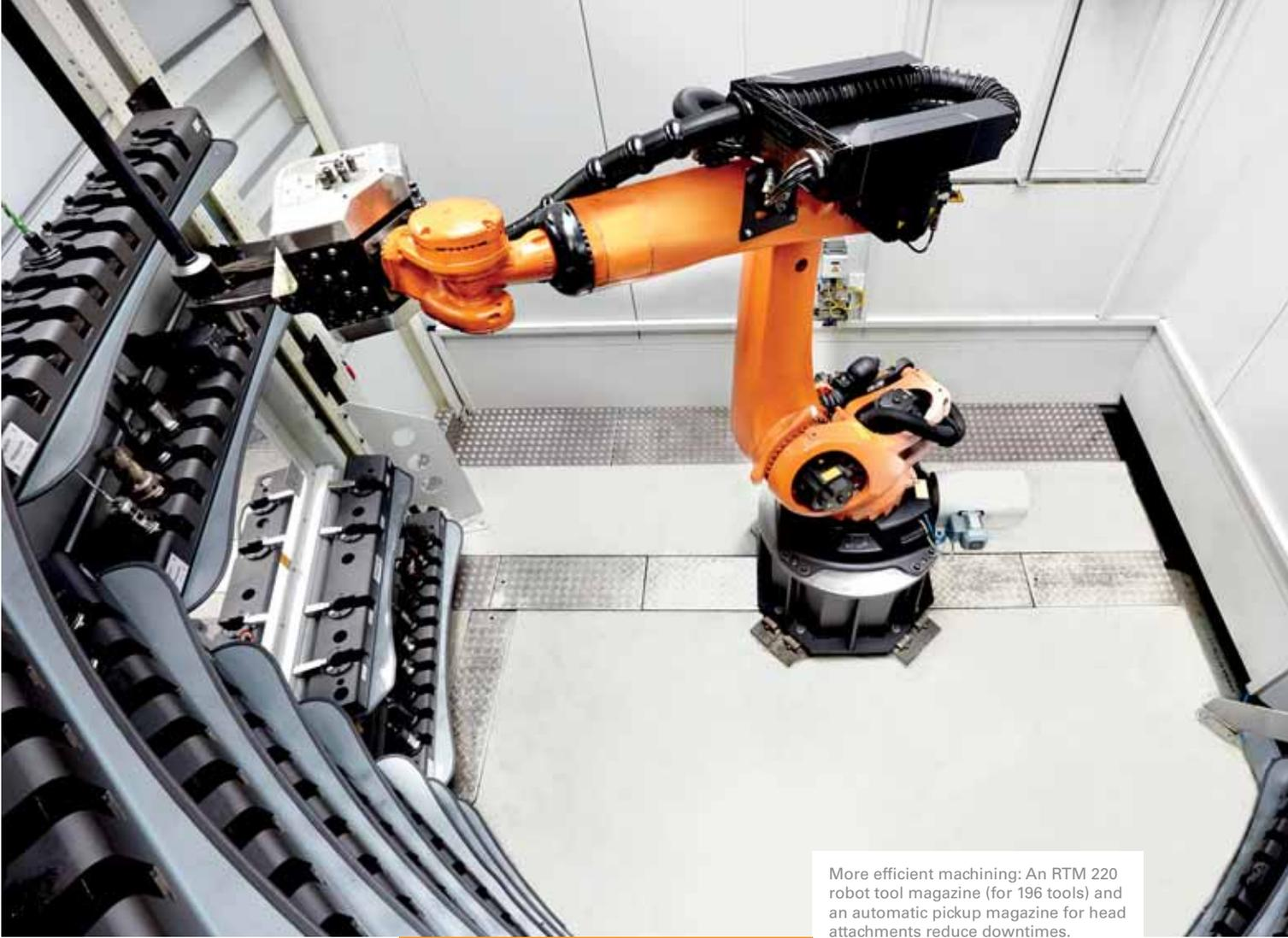
More efficient machining: An RTM 220 robot tool magazine (for 196 tools) and an automatic pickup magazine for head attachments reduce downtimes.
