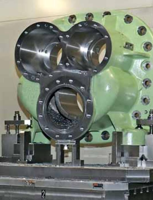
With an extended Z-axis and a machine table capable of supporting up to 2.5 tonnes, the Heckert HEC 800 Athletic is ideal even for the largest GEA Grasso housing.
