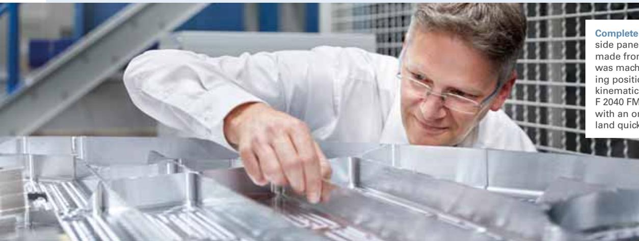
**Complete process:** This fuselage side panel for the Airbus A320, made from an aluminium blank, was machined in a single clamping position. Thanks to parallel kinematics, the ECOSPEED F 2040 FMS can even cut pockets with an only slightly inclined land quickly and elegantly.
