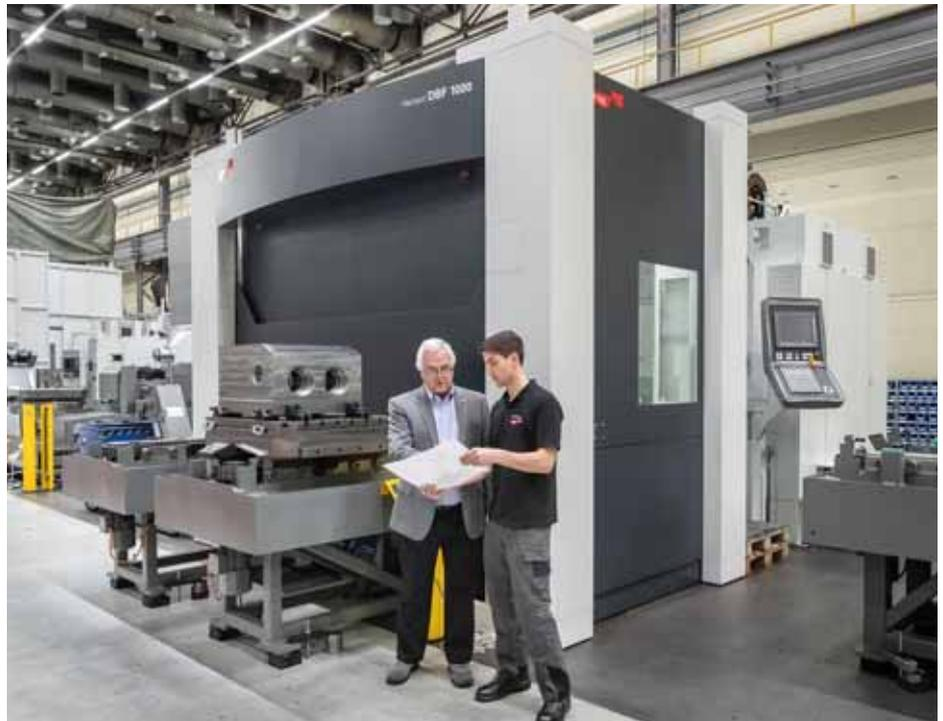
**Prepared for unmanned operation:** Thanks to the additional six-pallet linear storage and a 320-AC tool changer, the new Heckert DBF 1000 machining centre can also work without human intervention.
