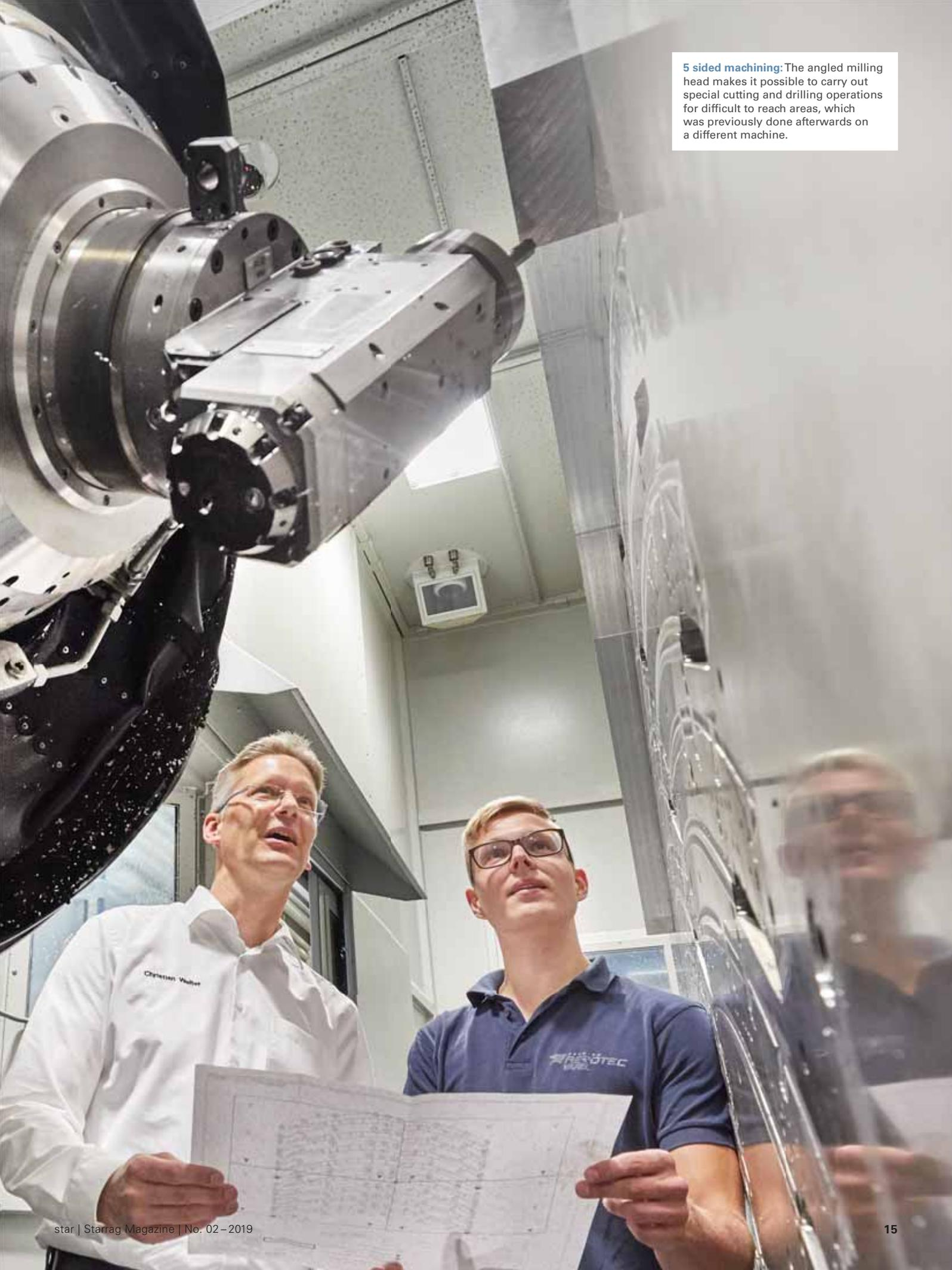
**5 sided machining:** The angled milling head makes it possible to carry out special cutting and drilling operations for difficult to reach areas, which was previously done afterwards on a different machine.
