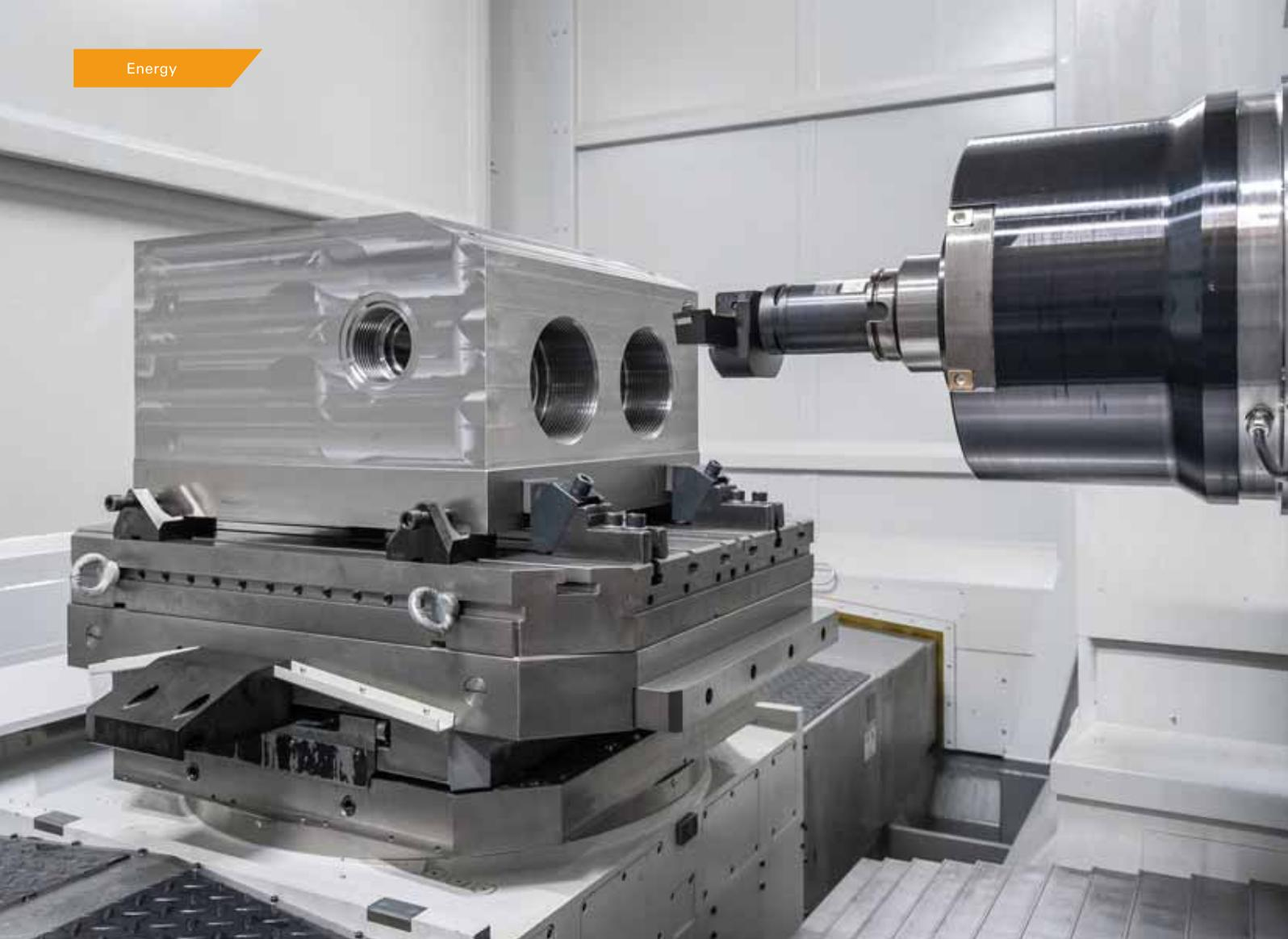
**“Heavy metal” in sight:** The new Heckert DBF 1000 machining centre is particularly suitable for highly efficient heavy-duty cutting of heavy housings weighing up to 4,000 kg, such as on the fluid ends.
