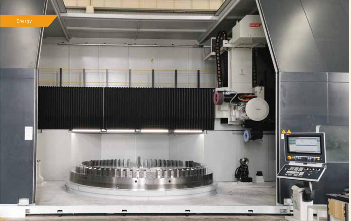
**Berthiez RVU 4700/450 with a 177.2 in. (4,500 mm) table diameter. On the new RVU grinding machines, it is possible to grind bearings of any size from 39.4 to 236.2 in. (1,000 to 6,000 mm) in diameter with micrometer precision.**
