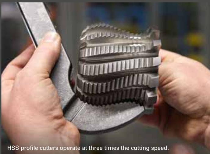
HSS profile cutters operate at three times the cutting speed.
