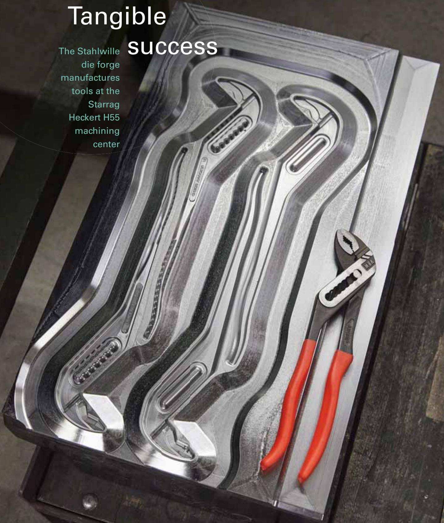
The Stahlwille die forge benefits from the precision and repeating accuracy of the Heckert H55 machining center
