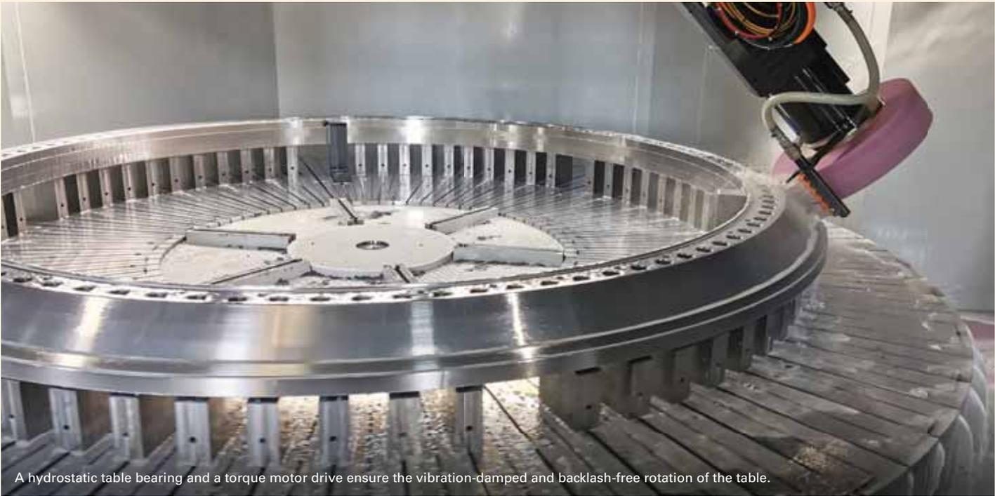
A hydrostatic table bearing and a torque motor drive ensure the vibration-damped and backlash-free rotation of the table.
