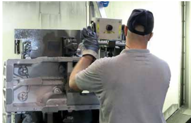
The loading station is completely opened to the top and allows an easy loading of the machine during primary processing time
