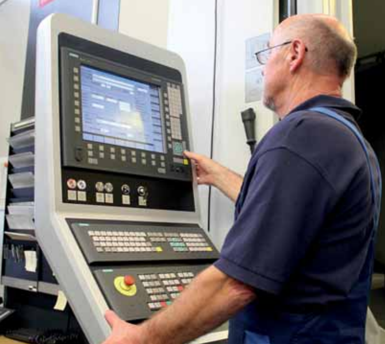
The Heckert HEC 630 Athletic horizontal machining centre is controlled by a Siemens 840 D sL. The CNC provides high ease of use, which the staff at CVS appreciate
