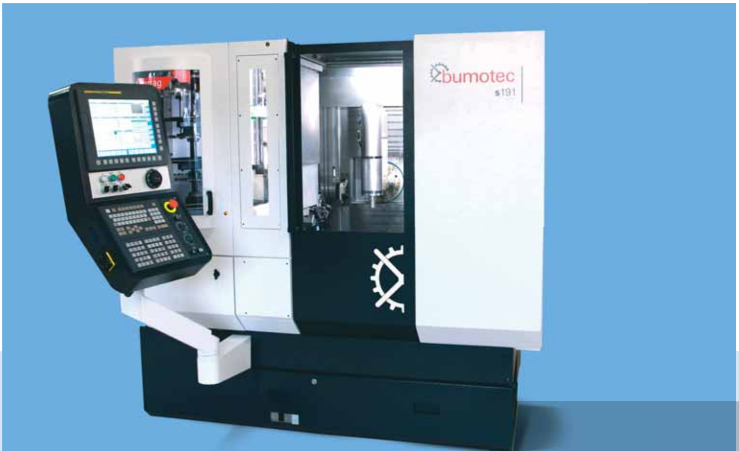
The S191H 16 linear CNC turn-mill centre is a proven solution for the six-sided complete machining of components with backlash-free, repeatable precision in the µm range
