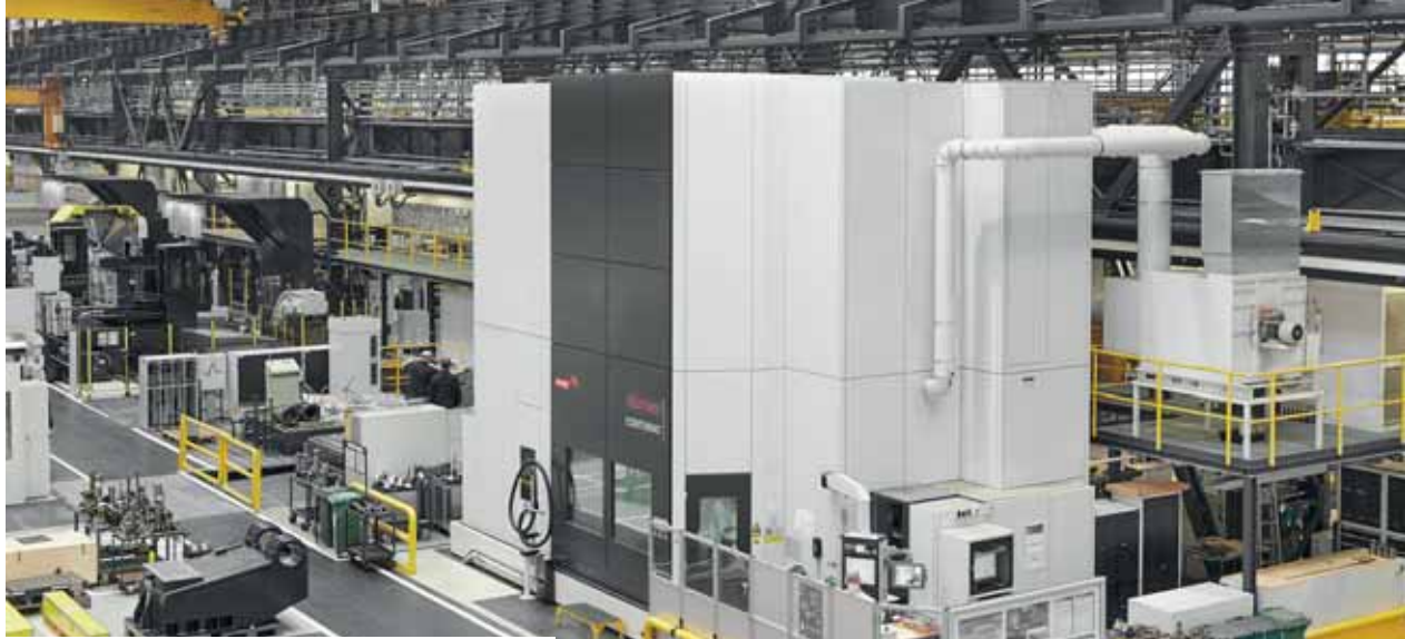
Towering: The seven metre-high CONTUMAT VC 2400 can be used to process workpieces weighing up to 17 tonnes, with a maximum height of 2,585 mm and a diameter of up to 2,400 mm
