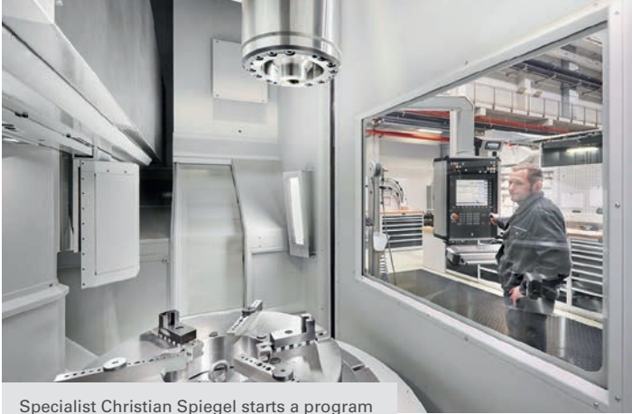
Specialist Christian Spiegel starts a program on the Dörries CONTUMAT that was created in a central programming department.
