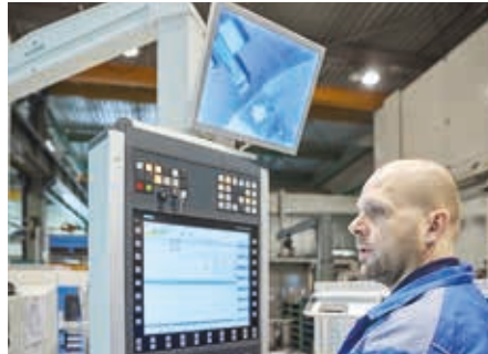
Always in the picture: Most of the machining work is done on the inner contour. Without the vision system, a worker such as Matthias Bauer would have little opportunity to observe the machining process in a completely enclosed machine.
