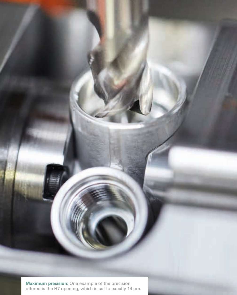
Ready for the ghost shift: Turned parts contractor Heinrich has put particular emphasis on a high degree of automation so that it can use the Bumotec s181 around the clock if necessary. For this purpose, the machine has been equipped with an automatic tool and workpiece change system.
