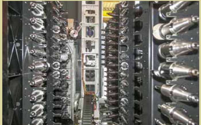
The tower magazine offers space for over 300 tools with a length of up to 800 mm.
