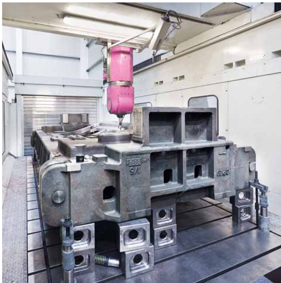
Premiere in East Westphalia: The first high-gantry machine for finishing and roughing was developed 19 years ago in Bielefeld as the Droop+Rein FOGS 32 55 M30 K.
