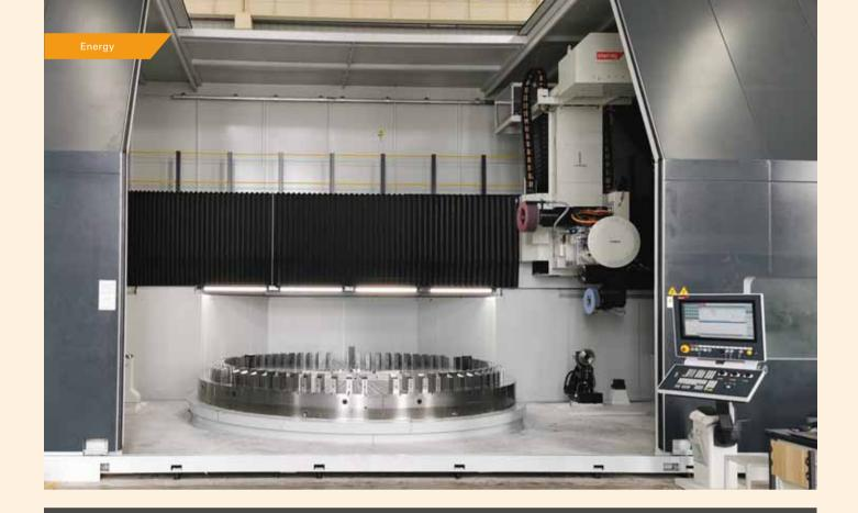
Berthiez RVU 4700/450 with a 177.2 in. (4,500 mm) table diameter. On the new RVU grinding machines, it is possible to grind bearings of any size from 39.4 to 236.2 in. (1,000 to 6,000 mm) in diameter with micrometer precision.
