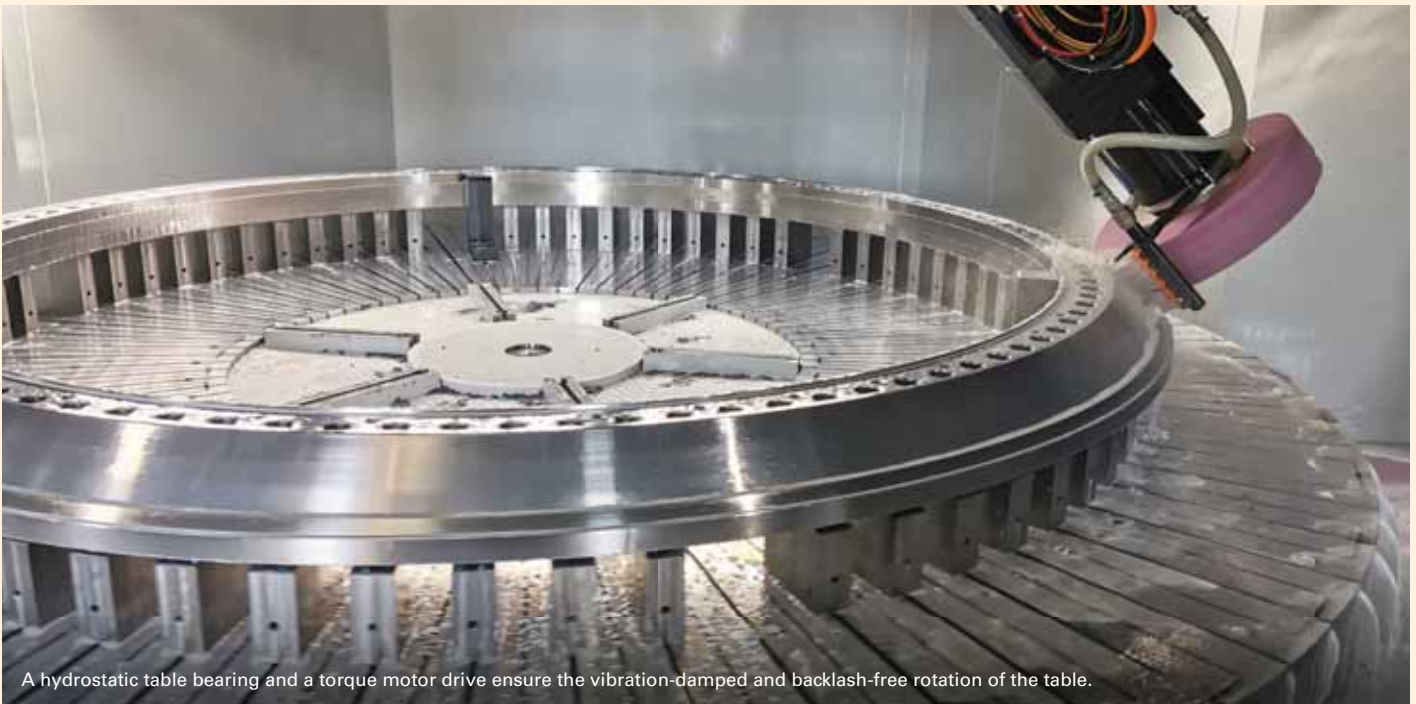
High-quality drive technology provides high machining accuracy.
