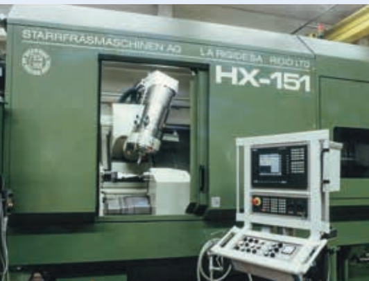
It’s all about the tempo: Starrag products aren’t just distinguished by their precision, but also by their productivity. One key example of this is this type HX-151 high-speed milling machine that was developed in the 1990s, which ABB uses to mill turbine blades.
