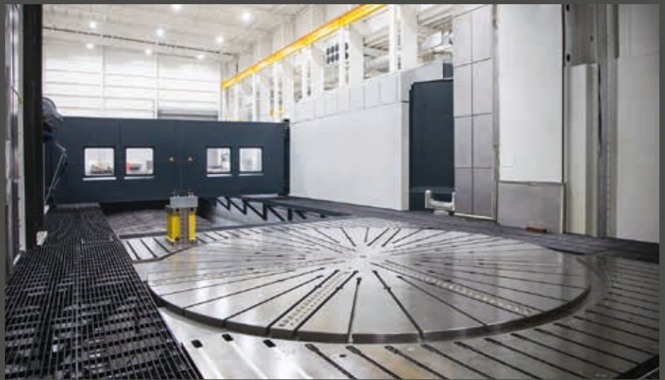
Heiko Quack: Everything, because you don't build a six-axis machine in these dimensions on a daily basis, with these milling and turning capabilities, with eleven machining heads, five tool systems and over 400 tools.
