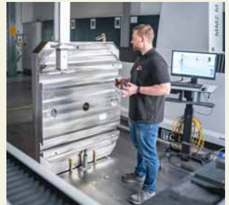
Decoupled from the measuring process – instead of just one station, there are four ZEISS programming workstations, where four experts create measuring programmes based on CAD data using the ZEISS CALYPSO programme.
