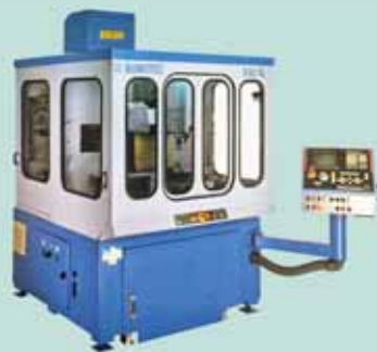
Bumotec S-92XL, 3- to 5-axis CNC in single- or multi-spindle configuration, produced in the early 1990s.
