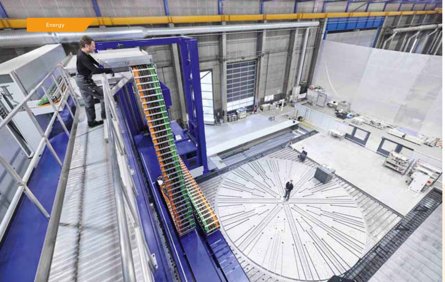
Half time: View from the bridge of the portal milling machine to the semi-transparent curtain, behind which the second portal turning machine is being built in 2024.
