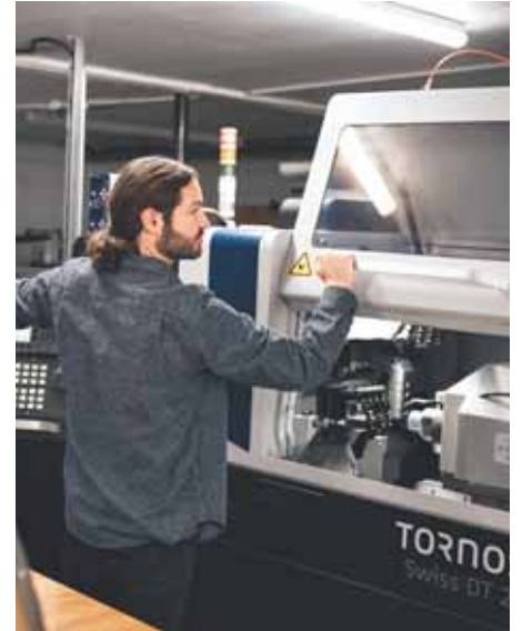
Weiss Watch Company's Tornos SwissNano and Swiss DT 26 (shown here) are equipped with bar feeders, providing founder Cameron Weiss a greater degree of autonomy.
