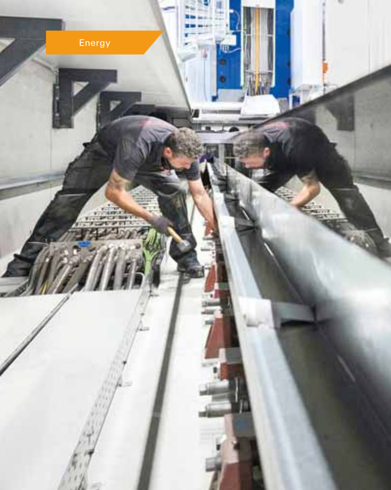
Sights set on XXL: The gantry axis of the portal milling machine moves over a distance of 46 ft (14 m).
