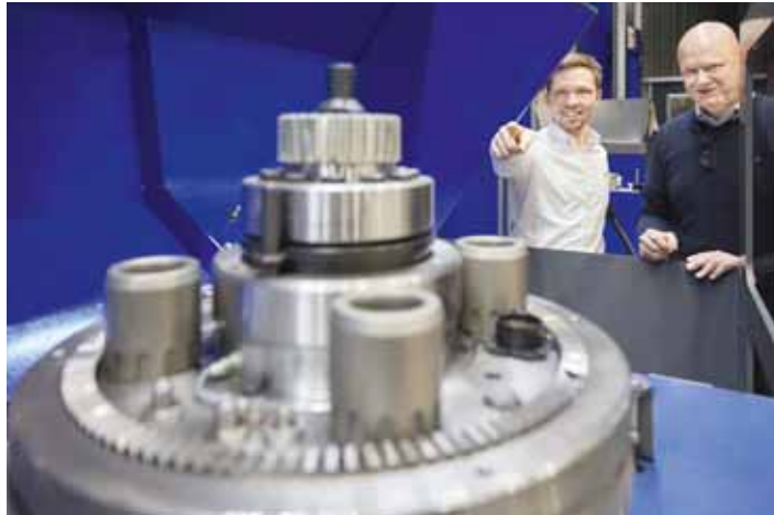
Fabian Schwarz (left), Head of Project Management LPMS (in conversation with HACO CEO Henning Albrechtsen): "Integration of the turning and milling processes enables production of complex workpieces with great precision and efficiency. This saves users time and money, as they need fewer machines and undergo fewer setup times."
