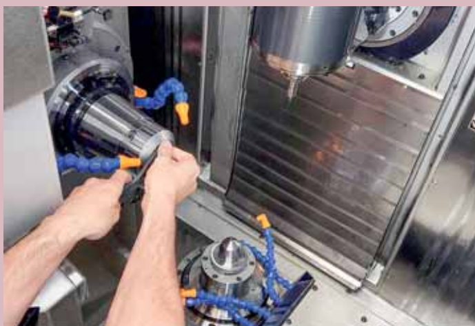
Adaptable: The large variety of parts requires particularly flexible machine kinematics with easy changeover, thanks to which the machining centers can be adapted to different production requirements without great effort.
