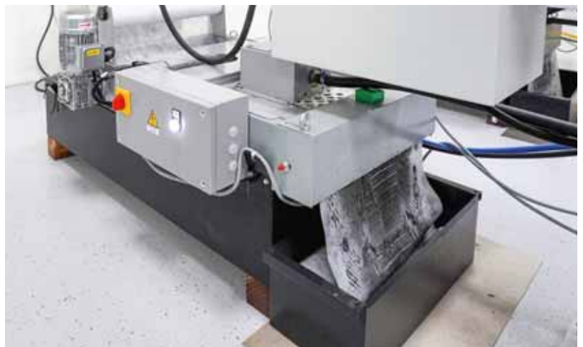
The paper belt filter system is one of the solutions that guarantees high process reliability.
