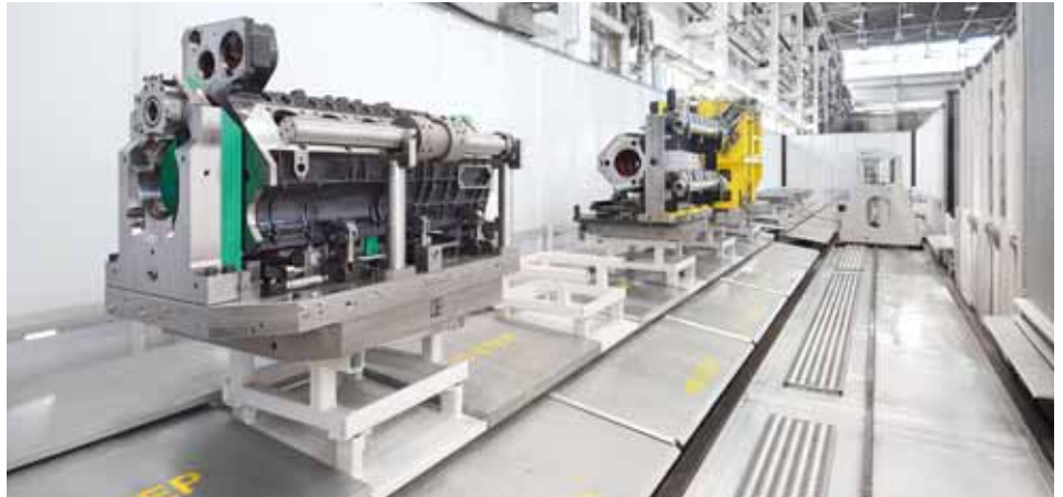
Tatra chose a pallet system as the automation solution, which initially contains twelve pallet spaces, and in a later stage 18 pallet spaces and a linear conveyor.
