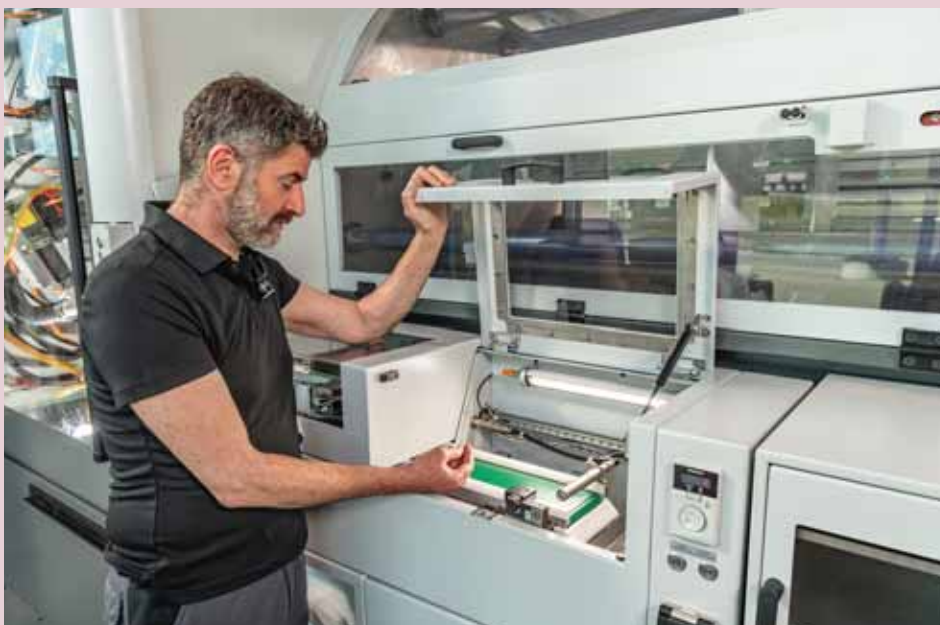
Easy access to the parts conveyor belt for quality control and unloading
