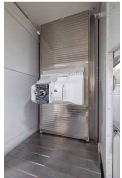
Starrag's own robust 53 kW gear spindle is used as a work spindle, which provides 1,600 Nm torque and a speed of 4,500 rpm.
