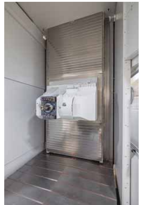
Starrag's own robust 53 kW gear spindle is used as a work spindle, which provides 1,600 Nm torque and a speed of 4,500 rpm.
